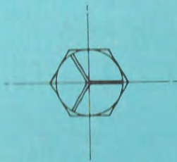
Fig 1 Bolt Identification Grade 5 Head Marking. U.T.S. 536 TON/in. 2 Threads to A.S. B18.2.
