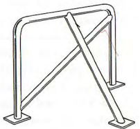
Type 3 Full Width Braced Roll Bar
