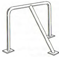
Type 2 Full Width Roll Bar
